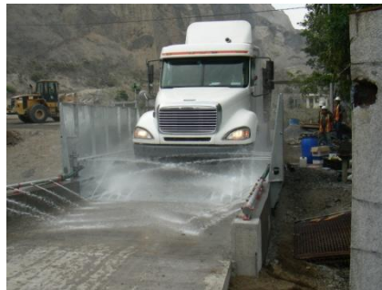
High Volume Low Pressure Focused Wash Water Delivery, Automatic Exit Area Wash Down
