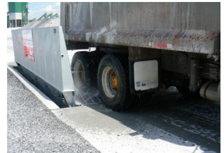
High Volume Low Pressure Wash Water Flow Through "Non Clog" Direct Tire Contact Nozzle System = Clean Tires & Roads / No Track Out
