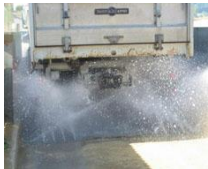
Intensive cleaning of the tyre profiles through the bottom nozzles
