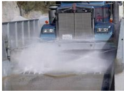
Intensive washing of the wheels, fenders and chassis
