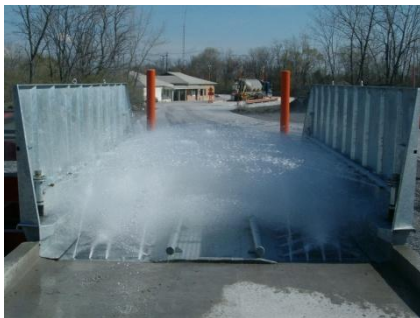
Focused high volume low pressure washing of wheels, fenders and chassis clean tires and roads.
