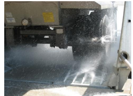
Close up direct nozzle to tire contact high volume water flow.
