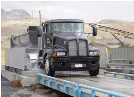
The 939's 3 –Tire Revolution & High Volume Focused Water Spray Delivers Clean Tires and Roads
