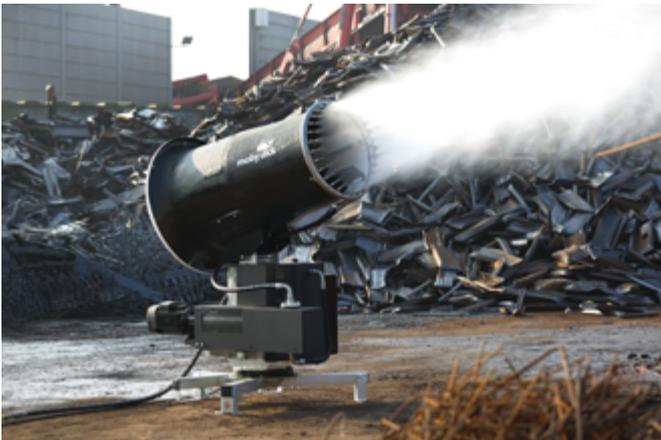
With their lower flight and rate of fall, they remain in the air longer and their suction effect is reduced, letting them bind more dust particles so that these can fall to the ground together with them. This technology has evolved into a proven system of dust control that makes manufacturing processes cleaner and satisfies labour protection regulations.
